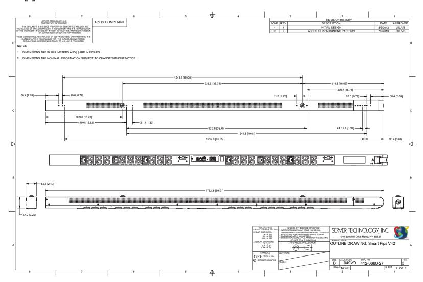
Zero-U Rack Mounted Cabinet PDUs with 42 Outlets
