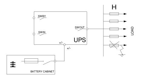
In order to select the correct protection devices to be inserted downstream of the MASTER HE, the following two operating modes have to be taken into consideration: *mains power supply* and *battery power supply*.
