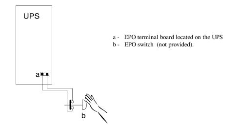
On the MASTER HE, the jumper on the EPO terminals (page 20) must be removed, and the wires from the auxiliary contact of the button must be connected in place of the jumper. The contact must be closed with the button in the rest position and must open when the button is pressed.
