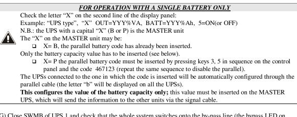
G) Close SWMB of UPS 1 and check that the whole system switches onto the by-pass line (the bypass LED on unit1 will flash while it must be on steady on the other UPSs), then open switch SWMB again. Wait a few seconds then check that the UPS1 returns to "NORMAL OPERATION".
