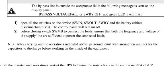
After all the maintenance operations, restart the UPS following the instructions in the section on START-UP PROCEDURE (see page 26). Then open disconnector SWMB (if it was previously closed). The MASTER HE will return to NORMAL OPERATION.
