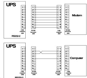
E - DB9 male marked RS232-2 For the modem connection use the RS232 standard cable. For the computer connection see the diagram.
