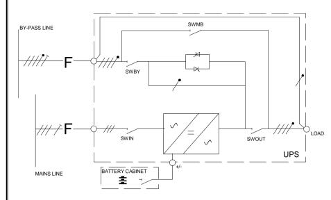
NOTE: The by-pass supply must be three-phase with neutral. *The UPS* cannot work without input neutral on the by-pass line (\*).
