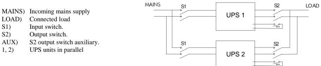
If circuit breakers are to be used the positions 1 and 2 adhere to the following:
